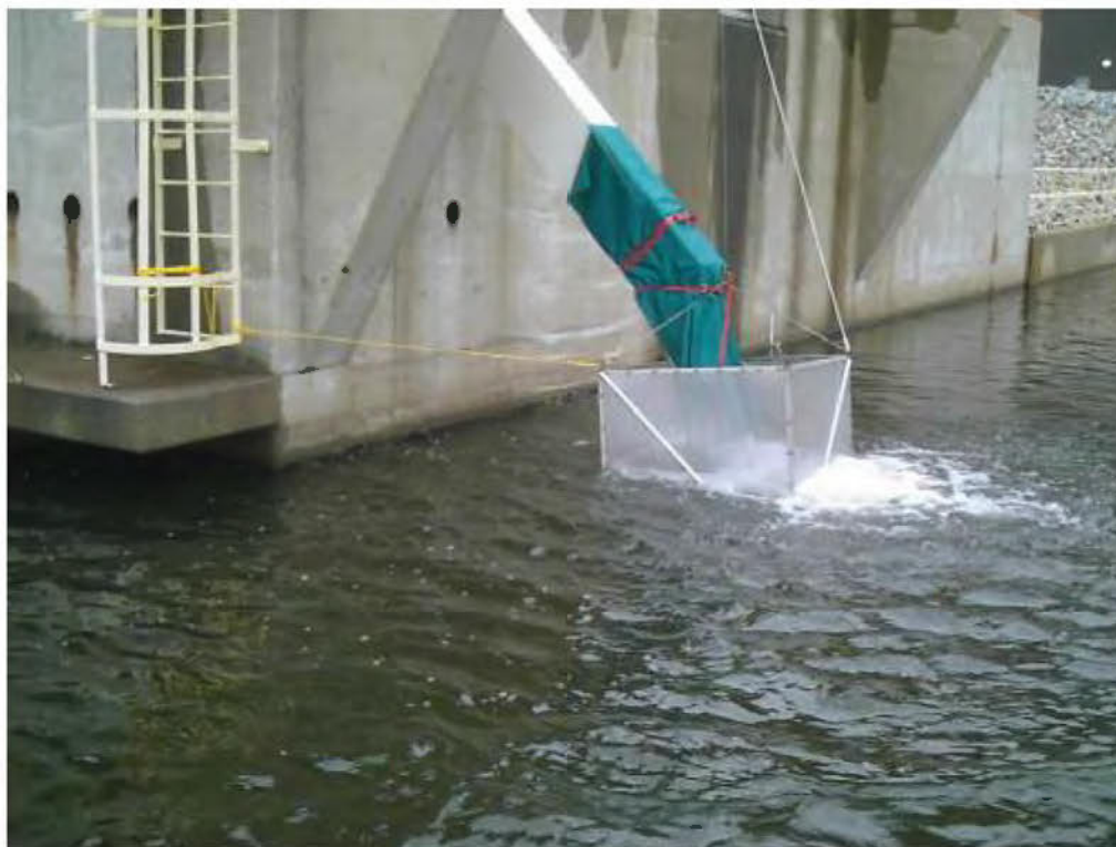
1. View of impingement sampling apparatus during pilot study screen wash.
